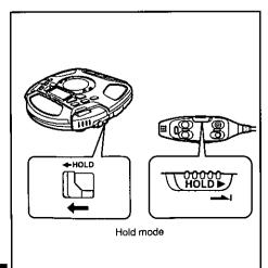
This function enables the unit to ignore accidental button presses. (The disc lid can still be opened and closed.)
